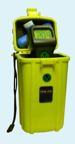
Standard package includes: TEK-OX Oxygen Analyser Quick-Ox Gas Sampling Kit R-17VAN Oxygen Sensor Waterproof Case 2 x AA Batteries
